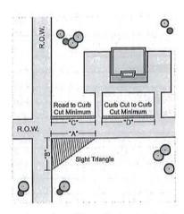
The following triangle segment lengths will apply to the determination of a clear sight triangle.
