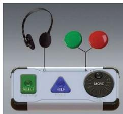
**Verity Touch Writer Duo** may be used with **Verity Access**, an Audio-Tactile Interface (ATI) intended for voters that cannot, or prefer not to, use the touchscreen. Verity Access includes two connection ports: the left connection port for headphones, and the right connection port for any dual-switch input device (such as tactile switches or sip-and-puff devices).
